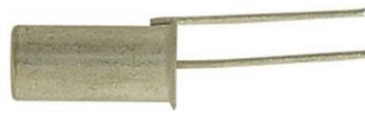
Tilt switch When tilted a ball bearing bridges the contacts inside, completing the circuit.
